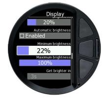
Press middle button to enter edit mode. Slider background colour will change to white. Use upper and lower button to increase or decrease value. Long press will make a bigger increase or decrease. Confirm selection with short press on middle button. Long press middle button to cancel selection and exit without changes.
