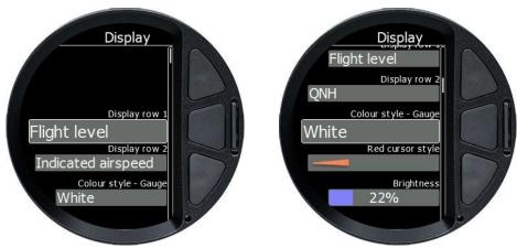
**Display row 1 and Display row 2** are used to select values which are shown in top row or bottom row. User can select among following options: QNH, Battery voltage, Outside temperature, Vertical speed, Density altitude, Flight level, Height above take-off elevation, Altitude, True airspeed, Indicated airspeed and none.
