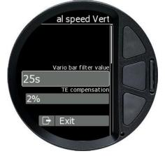
TE compensation is used mainly for gliders in order to show total energy change rather than vertical speed. Set to 100%, if you want to have compensated vertical speed indication or leave on 0 to have non-compensated vertical speed.
