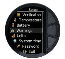
When you press middle button for longer time, you will get into setup menu. Press upper and lower button to move focus. Quickly press middle button to enter submenu. Long press middle button to exit submenu or select Exit option in menu.
