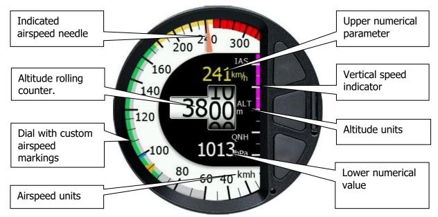
In the middle of screen altitude is displayed as rolling counter. On the right side vertical speed is drawn as a magenta bar. Additionally, two numerical values can be show. See chapter 5.3.1 how to customize main screen.
