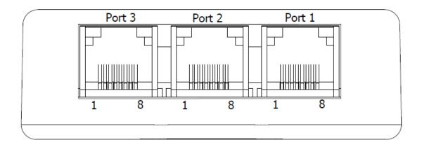
FlarmACL connects together Pin 1 from Port 1-3, Pin 2 from Port 1-3, etc. Pin names are:
