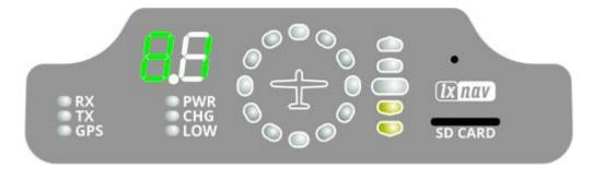
On picture below is code 81, which means No Obstacles.
