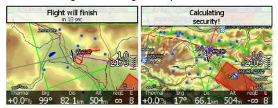
The flight is finished when the message Calculating security disappears. At that moment the statistics page will be changed back to logbook view. Now it is safe to switch off the instrument.
