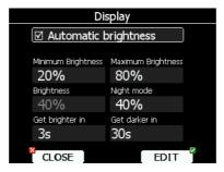
If the **Automatic brightness** checkbox is selected, the instrument will automatically adjust brightness according to current light conditions. **Minimum** and **Maximum brightness** items control value limits. Use time values to setup how fast adaptation to brighter conditions or darker conditions will occur. Default values are tuned to human eyes and do not require change.
