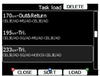
Total task distance, task description and task points are shown for each task stored. Select the desired task by rotating the lower-right knob and press **LOAD**. The task will be loaded into the active task and the task edit dialogue will be opened.
