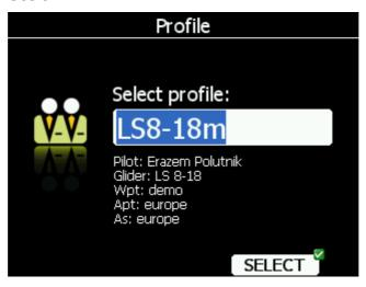
Turn the lower-right knob to select the desired profile if more than one profile is available. For the selected profile the pilot name, glider type, loaded way point files, loaded airports databases and loaded airspace databases are shown.
