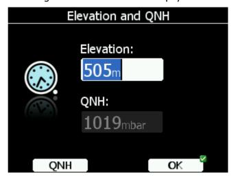
The instrument will offer elevation from the terrain database based on current latitude and longitude. Elevation will mostly be within few meters from the current elevation. Use the lower-right knob to fine-tune the elevation.
