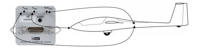
If the unit is to be configured for pneumatic TE compensation using a TE tube, then the connections are:
