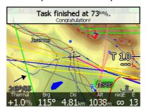
If you want to fly a new task without landing, load the new task and press the **RESTART** button.
