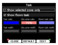
**Task colour** defines the colour of task lines. **Obs.zone colour** defines colours for observation zones. Use the lower-left knob to change transparency of area. 100% means completely transparent and only the outline will be drawn. 0% means completely solid (not recommended). When **Show flown task** is checked also the flown task will be drawn. This might be useful when flying assigned area tasks.
