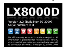
In two-seat gliders it is possible to install the LX8000D rear seat device. The LX8000D looks almost identical to the LX8000. However inside the device there is no GPS or Flarm module. The rear seat device must be connected only to the LX8000 via the RS485 bus system. Power is available from the bus hence no external power is needed. The device can be switched on only when the LX8000 is powered on.
