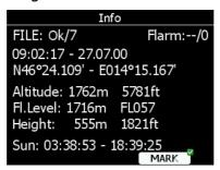
If you press the **MARK** button a new way point will be created with the current latitude, longitude and elevation based on the terrain database. The way point name is generated from the current date and time separated by the minus character and preceded by an underscore.
