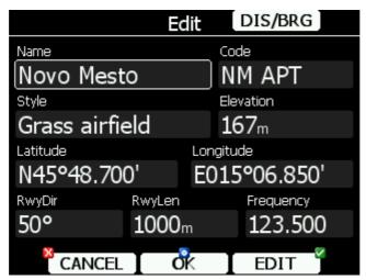
There are two possibilities to enter a position. You can modify latitude and longitude to define a position of the point or press the **DIS/BRG** button to enter the position as distance and bearing to a selectable point.
