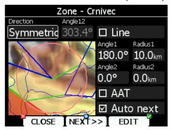
Using parameters in the zone dialogue it is possible to describe all types of observation zones. **Angle12** defines the orientation of the observation zone. Available parameters for **Direction** are:
