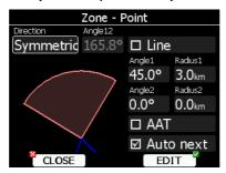
Using parameters in the zone dialogue it is possible to describe all types of observation zones. **Angle12** defines the orientation of the observation zone. Available values for **Direction** are:
