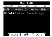
The list is sorted by distance. Select the desired Flarm target and press the **GOTO** button. You will start navigating to this Flarm position. Instead of Flarm device ID you can also
