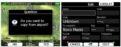
The minimum data that must be entered are name, latitude and longitude. Press the **OK** button to confirm changes and create the new way point. The new way point is added to active way point file. Press the **CANCEL** button to abandon creation of new point.
