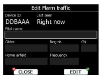
Enter data about the Flarm glider and pilot. The LX8000 is pre-loaded with the FlarmNet database to identify known FLARM Device IDs with plane and pilot data. You can upload the latest FlarmNet database after downloading it from <a href="http://www.flarmnet.org">http://www.flarmnet.org</a>. The update procedure is similar to the update procedure for airport databases. See Chapter 5.1.5.2 for more details about updates.
