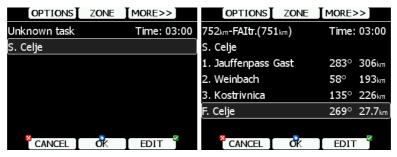
Move the cursor down to the next empty point and repeat the above procedure until the entire task is entered.
