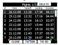
If a SD card or USB stick is inserted into the LX8000, flights can be copied to it when the corresponded button is pressed. Flights can be removed from the LX8000 using the **DELETE** button.
