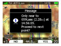
A message will appear. If you confirm this with **YES** the task will be advanced to the next turn point and it will recalculate the task taking the optimal fix as the task point.
