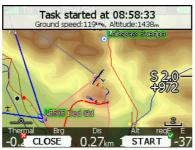
Ground speed and pressure altitude are also shown in the message. At the bottom two buttons are displayed. Use the **CLOSE** button if this was not a valid start and you want to remove the message from screen. If message is removed it will appear again next time you leave the start zone. If you press the **START** button navigation will be advanced to the first turning point.
