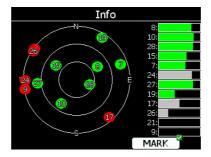
Green satellites are satellites currently being used for position determination. Three concentric circles represent satellite elevation (0, 30, 60 degrees above horizon). If a satellite is in the centre of the circles it is directly overhead.
