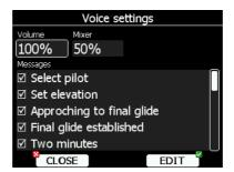
In the **Voice settings** menu volume level (loudness) of the voice module and mixing level between voice and vario sound can be adjusted. In the Messages window each item can be set separately. Only checked items will be posted to the voice module.
