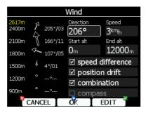
The wind profile is shown on the left side of the dialogue. Yellow coloured altitude indicates our current MSL altitude. Using the lower-left knob you can scroll up and down through the wind layers.
