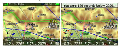
The lower number shows the difference to the set altitude. Negative values mean altitudes below set altitude. The upper yellow number indicates the number of seconds left to be below the set altitude. Chevrons indicate meters below or above required altitude. Each line represents 10 m. A message "You were XX seconds below YYYYm!" is displayed once you fulfil the conditions.
