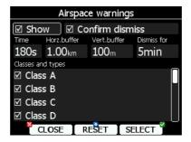
Airspace warnings are the most complex ones. An airspace warning is activated by two triggers; First warning (orange) will be given when a projected position of flight for period, which is defined in the **Time** item, is computed to cross an airspace zone.
