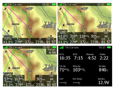
The first page is identical to first pages of the airport and way point modes. It shows navigational data to the current turn point. However the final glide indicator always shows the required altitude to complete the task.
