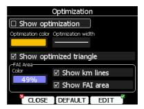
Check the **Show optimization** item to enable display of the optimised track. **Optimization colour** and **width** defines the colour and width for these lines.
