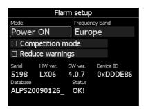
**Device ID** shows the Flarm unique ID, which is transmitted to other FLARMs. The Flarm status message is normally OK. In case of any errors or warning an error message will appear. The user can change the operation mode of Flarm unit, frequency and enable/disable competition mode.
