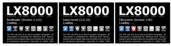
The boot procedure normally takes 15 seconds but in the case of a firmware update or system check it can take more time. The final boot screen displays information about the LX8000 firmware and the IGC serial number.
