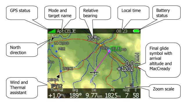
In the top row the GPS status is shown. Green colour represents GPS 3D, yellow colour means GPS 2D and red colour is GPS bad. The number of coloured bars indicates the number of visible satellites. Each bar represents two satellites.
