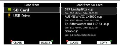
In next step the data source must be selected. A dialogue with a list of all available files will be opened. Press the COPY button to copy the selected file to the LX8000. The LX8000 will accept the following file formats:
