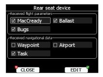
Data are divided into two groups; flight parameters and navigational data. If a specific value is checked this value will be automatically received from the other device.
