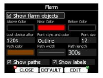
Checking **Show Flarm object** will enable display of aircraft detected by FLARM.
