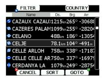
Press the **SORT** button to change the sort order of the airports. Select an airport using the lower-right knob. Press **GOTO** and you will navigate to it.
