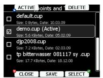
Multiple files can be selected. All checked files will be shown on the graphics page and used in the near mode calculation, if the way point is of the proper type (airport or outlanding
