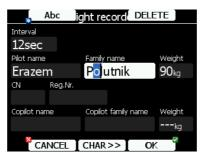
Press the **CHAR>>** button to advance the cursor to the next position. The cursor can also be moved to next position using the bottom-left knob. Rotate it clockwise to move forward.
