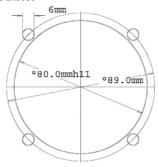
Prepare the cut-out in the instrument panel according to the drilling template. Remove the press-in covers from the four main rotary switches on the LX8080. While holding the knobs, slacken the screws with a screwdriver. Now the knobs can be removed (never use power to remove the knobs, you can damage rotary switches). Remove the four M6 screws. Position the LX8080 in the cut-out in the instrument panel. Tighten the LX8080. Tighten the knobs and fix the covers
