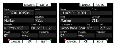
Way point data can be modified. Refer to Chapter 5.6.1 for more details. Press the **OK** button to save a marked way point or press **CANCEL** to exit without saving. Press **GOTO** button to navigate immediately to selected point.
