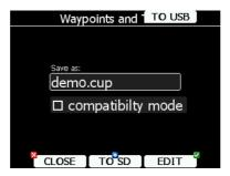
Change the filename if required. Press **TO USB** for saving to the USB stick or press **TO SD** for saving to the SD card. When the compatibility mode flag is checked the file will be saved in DA4 format, which can be used with older LX devices (LX20, Colibri, LX5000, and LX7000).
