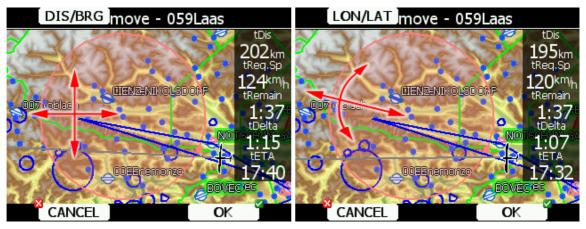
In the upper-right corner the remaining task distance, required task speed, remaining task time, delta time and estimated time of arrival are shown.
