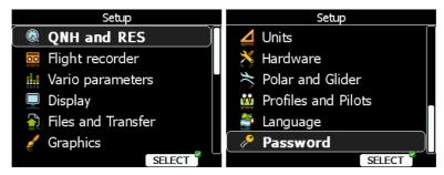
The setup menu is slightly different on the rear seat device as not all options are applicable. Items which are marked with an asterisk (\*) are available only in the front seat setup menu.
