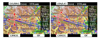
In the upper-right corner the remaining task distance is shown as well as the required task speed, remaining task time, delta time and estimated time of arrival.
