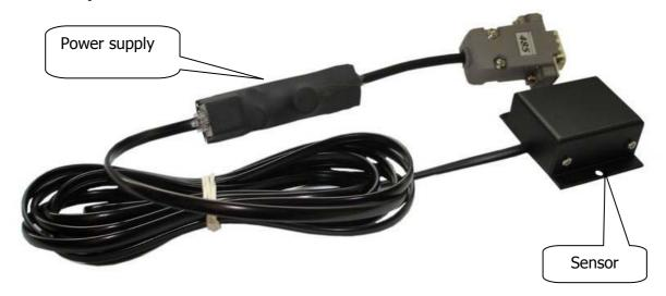
The compass module is an electronic compass device (magnetic field sensor) which was developed for the LX8000. The LX8000 recognises the compass module automatically when it is plugged into the RS485 bus. The only configuration settings needed are related to the compensation procedure. An indication that the compass module is connected is the appearance of raw data readings in the compass calibration page.
