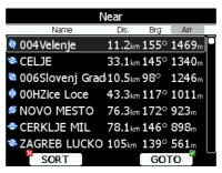
Select the preferred landable place via the lower-right knob and press the **GOTO** button. It will automatically change to airport mode and navigation will commence to selected point. Duplicates are automatically removed. If a target with nearly the same latitude and longitude is found within both the distributed airports database and user way point file then only the target from the user way point file will be displayed.
