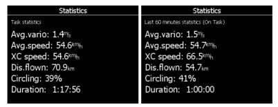
• The **last 60 minutes** statistics displays data for the last 60 minutes of flight. If the task was started then **Dis.flown** is the distance flown on the task for the last hour otherwise it is the optimised distance. If the task distance is used a remark (On Task) is displayed in the header.
