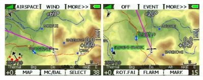
Press the **MORE>>** button to see more options. If the remote stick is available the behaviour is slightly different. When the check button is pressed on the remote stick a menu will appear instead of the button functions.
