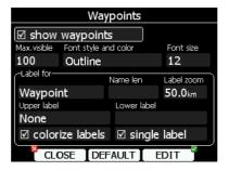
The **Max.visible** item defines how long way point labels and detailed symbols are shown. If the maximum number of way points on the current screen is more than the defined value only small blue dots will be shown for way points and no labels will be drawn.
