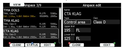
The VIEW button toggles the list views. When the **STATUS** button is pressed the status of the selected airspace zone will toggle between **OFF always**, **OFF today**, **OFF hh:mm** and enabled.
