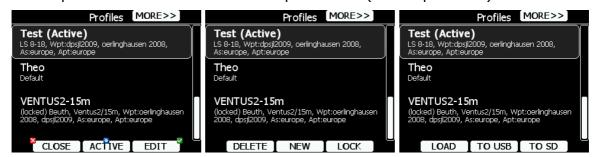
Use this dialogue to add a new profile, delete a profile, load/save a profile, change name for an existing profile and to activate a profile. The active profile is the profile which is currently being used.
