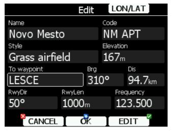
Press the **LON/LAT** button to toggle back to input of latitude and longitude. Modify other attributes at your discretion. When finished press the **OK** button to confirm changes or press **CANCEL** to dismiss changes. The modified way point will be updated in the appropriate file automatically.
