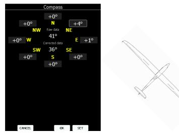
4. Stabilise the reading and press **SET** to save the correction for this direction.
