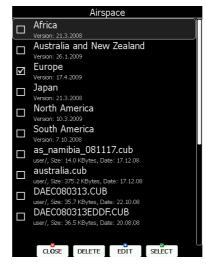
Select the required airspace and press **SELECT**. If a check mark is shown in front of an airspace item, this airspace file will be shown in the graphics and used for proximity calculation, when enabled.
