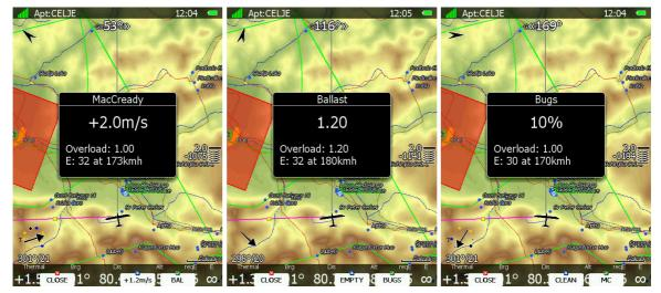
Use the lower-right knob to modify the MacCready setting. In the middle button there is a suggestion for the MacCready setting which is based on the last four thermals. Additionally to the selected MacCready value an overload factor is also shown together with the calculated glide ratio with corresponding speed.
