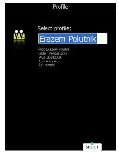
Turn the lower-right knob to select the desired profile if more then one profile is available. For the selected profile the pilot name, glider type, loaded way point files, loaded airports databases and loaded airspace databases are shown.
