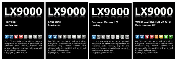
The boot procedure normally takes up to 20 seconds but in the case of a firmware update or system check it can take more time. The final boot screen displays information about the LX9000 firmware and the IGC serial number. When the boot procedure is completed the profile selection dialogue is shown. Please refer to Chapter 7.1 for more details about starting up the LX9000.
