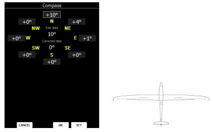
2. Stabilise the reading and press **SET** to save the correction for this direction.
