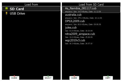
In next step the data source must be selected. A dialogue with a list of all available files will be opened. Press the COPY button to copy the selected file to the LX9000. The LX9000 will accept the following file formats:
