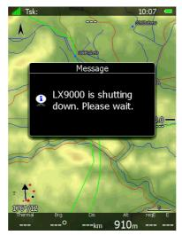
The LX9000 can also be powered off by pressing the upper-left button until the message "switching off" appears.
