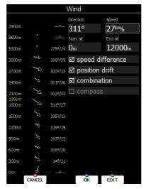
The wind profile is shown on the left side of the dialogue. Yellow coloured altitude indicates our current MSL altitude. Using the lower-left knob you can scroll up and down through the wind layers.
