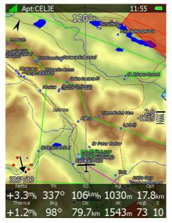
The additional items are the current net vertical speed, current track, ground speed, height above ground and optimised distance.
