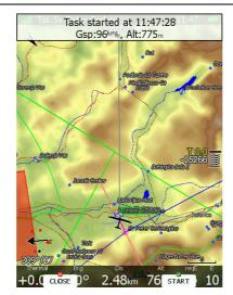
Ground speed and pressure altitude are also shown in the message. At the bottom two buttons are displayed. Use the **CLOSE** button if this was not a valid start and you want to remove the message from screen. If message is removed it will appear again next time you leave the start zone. If you press the **START** button navigation will be advanced to the first turning point.
