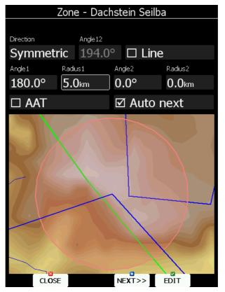
Using parameters in the zone dialogue it is possible to describe all types of observation zones. **Angle12** defines the orientation of the observation zone. Available parameters for **Direction** are:
