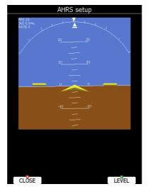
Place you glider in levelled position and press LEVEL button. You can also modify pitch only, if you rotate PAGE UP/DOWN rotary knob.
