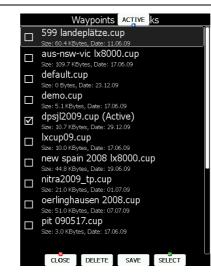
Multiple files can be selected. All checked files will be shown on the graphics page and used in the near mode calculation, if the way point is of the proper type (airport or outlanding place). However, only one file can be the active file. The active file is used for task creation.
