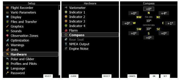
1. Orient the glider to face north. The **N** label will be automatically highlighted.
