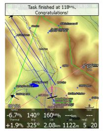
If you want to fly a new task without landing, load the new task and press the **RESTART** button.
