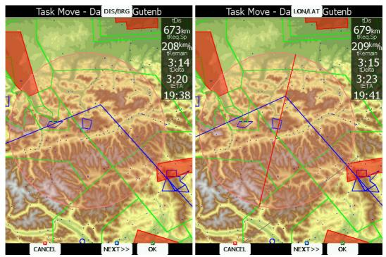
In the upper-right corner the remaining task distance, required task speed, remaining task time, delta time and estimated time of arrival are shown.
