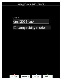
Change the filename if required. Press **TO USB** for saving to the USB stick or press **TO SD** for saving to the SD card. When the compatibility mode flag is checked the file will be saved in DA4 format, which can be used with older LX devices (LX20, Colibri, LX5000, and LX7000).
