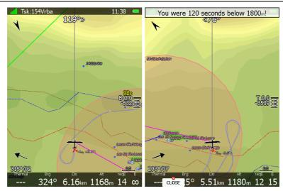
The lower number shows the difference to the set altitude. Negative values mean altitudes below set altitude. The upper yellow number indicates the number of seconds left to be below the set altitude. Chevrons indicate meters below or above required altitude. Each line represents 10 m. A message "*You were XX seconds below YYYYm!*" is displayed once you fulfil the conditions.
