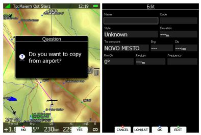
The minimum data that must be entered are name, latitude and longitude. Press the **OK** button to confirm changes and create the new way point. The new way point is added to active way point file. Press the **CANCEL** button to abandon creation of new point.
