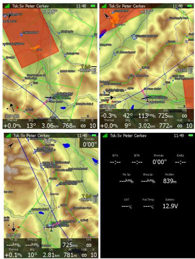
The first page is identical to first pages of the airport and way point modes. It shows navigational data to the current turn point. However the final glide indicator always shows the required altitude to complete the task.
