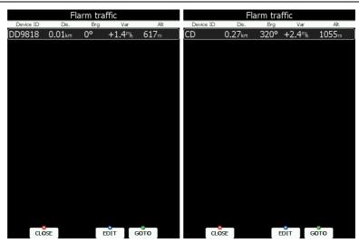
The list is sorted by distance. Select the desired Flarm target and press the **GOTO** button. You will start navigating to this Flarm position. Instead of Flarm device ID you can also show the competition number for a particular glider. Press **EDIT** to enter the edit dialogue for the selected Flarm object.
