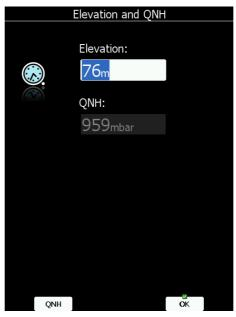
The instrument will offer elevation from the terrain database based on current latitude and longitude. Elevation will mostly be within few meters from the current elevation. Use the lower-right knob to fine-tune the elevation.
