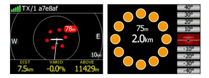
A warning can be dismissed with a short press of any button. Dismiss time can be configured in setup.
