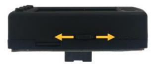
Moving the rocker button will increase or decrease the sound volume when on an info page. On pages with the map, the rocker button has a zoom function.
