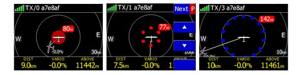
All targets are displayed as a glider symbols. It's also possible to change the object's colour, depending on the relative altitude to our position. All received targets (Flarm or PCAS) are marked with the same type of symbol except undirected targets, for which we don't know from which direction they are coming from. Flarm targets can be separated only by their ID.
