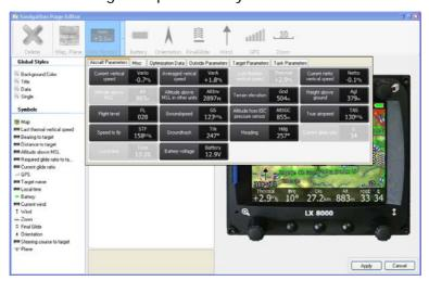
Data symbols are grouped in six groups: aircraft parameters, outside parameters, target parameters, task parameters, optimization data and misc tab. More details about data symbols on particular tab are given in chapter 3.2.2.
