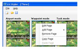
Select appropriate menu item to add, remove, copy or edit page. You can also drag page to another location. Press left mouse button and while holding it down, drag selected navigational page to desired location. A red line will indicate new position of page. Release mouse button to place page.
