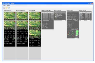
The main window consists of menu, toolbar and main view, where all seven LX8000 navigational modes are shown, namely airport mode, waypoint mode, task mode, statistics mode, setup mode, info mode and near mode.
