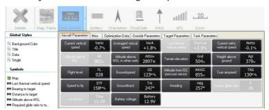
Data symbols are grouped in six logical groups: aircraft parameters, outside parameters, target parameters, task parameters, optimization data and misc tab.
