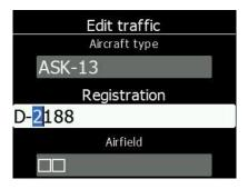
Pressing the **right push button** will move cursor right. **Left push button** will move cursor left. At last character position, right push button will confirm edited value, long press to **rotary push button** will cancel editing and exit that control. **Middle push button** will delete selected character.
