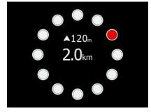
If modern view is chosen, warnings will be displayed as 3D visualisation of the approaching threat. This is for the highest alarm level (level 3) and indicates that impact is 0-8 seconds away. Example picture shows us an airplane approaching us from front left (11 o'clock) 40m below us. This screen will only display if airplane is approaching head-on (from the front).
