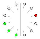
**Note:** Head-on  $(\pm 15^{\circ})$  traffic and collision warnings on Classic FLARM F6-F9 are indicated as shown in the graphic below (the traffic in this example comes from  $+5^{\circ}$  relative bearing).
